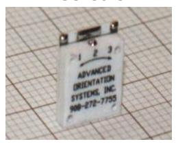
SX-070D-LIN, SX-030D-LIN and SX-015D-LIN are single axis LINEAR ceramics based electrolytic tilt sensors provide economical and reliable single tilt axis solutions for applications where very good linearity, high resolution and superior
